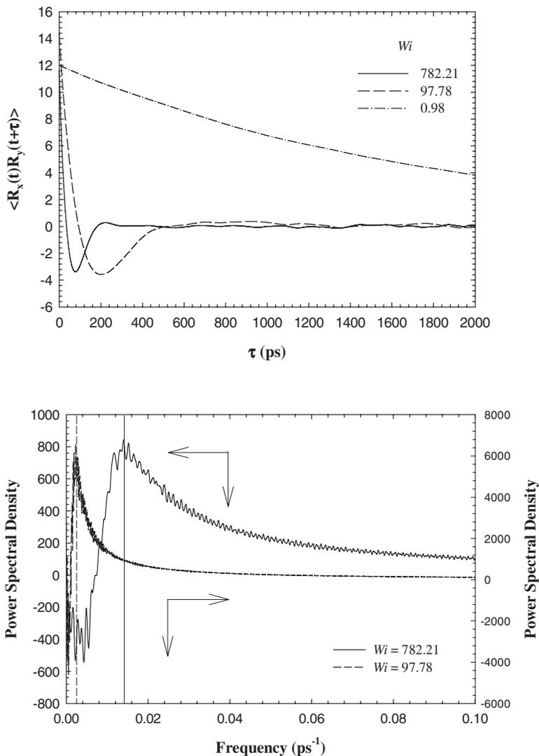
**FIG. 9.** Time cross-correlation functions versus observation time for three values of  $Wi$  and the power spectral density versus frequency for two values of  $Wi$  that exhibit minima in the cross-correlation function curves in the dense liquid simulations.
