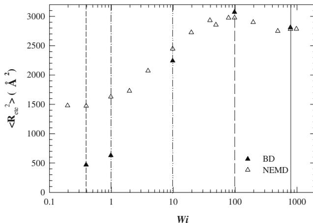
**FIG. 2.** The mean-square chain end-to-end distance,  $\langle R_{ete}^2 \rangle$ , for  $C_{78}H_{158}$  as a function of  $Wi$  from the atomistic NEMD (open symbols) and BD (filled symbols) simulations.
