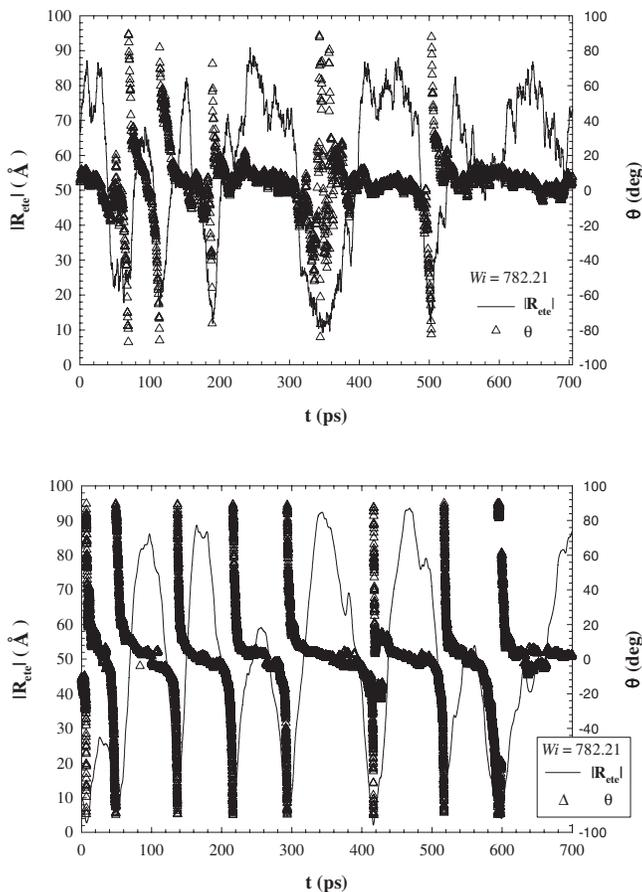
**FIG. 5.** The magnitude of end-to-end vector,  $|\mathbf{R}_{ete}|$ , and the orientation angle with respect to the flow direction,  $\theta$ , as functions of time for a random chain of the (a) NEMD and (b) BD simulations.
