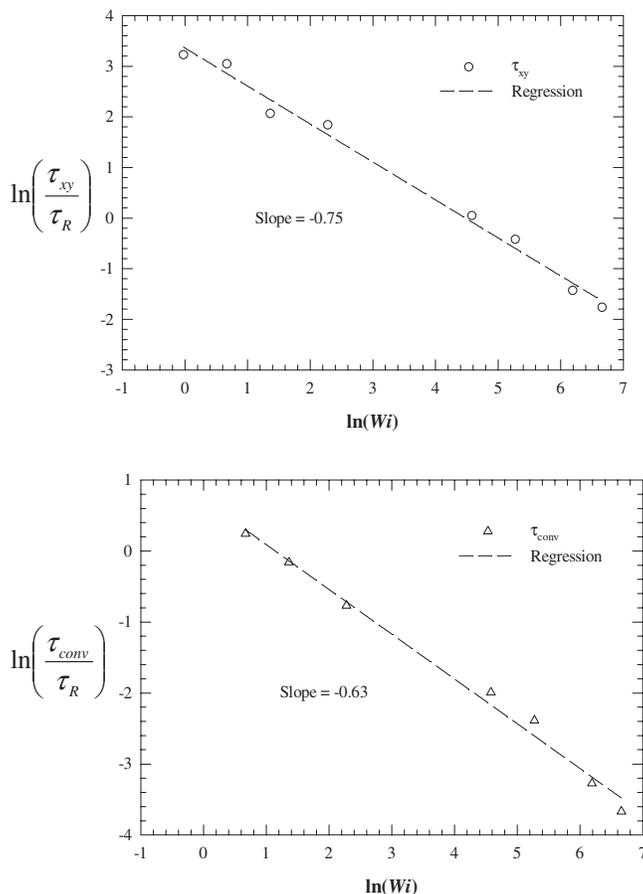
**FIG. 11.** Log-log plots of the characteristic time scales, relative to the Rouse time, versus  $Wi$  for the NEMD simulations. Note that plots of the characteristic frequencies would possess slopes of opposite sign but of the same absolute values as those presented in the figures.
